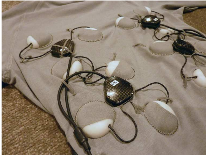
Haptic motor modules with carbon fibre variant.
