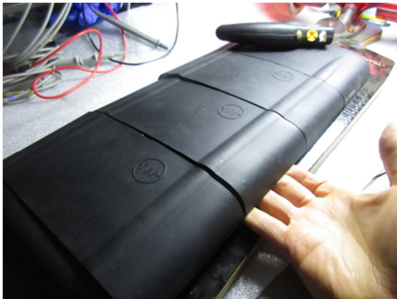
Massive battery flex, twist and gaps... still functioning.
