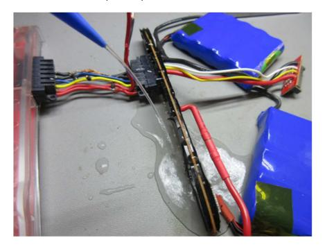
Fitment was good. A slight over-fill on the rear caused some minor interference with the 3 screw bosses. Although it fit the enclosure with some minor flex, over-fill is difficult to control to prevent fitment issues.
