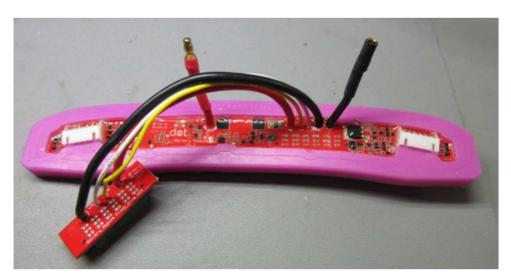
The PCBA below is resin coated with a clear material. Hard to see in the picture.
