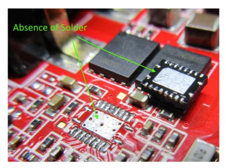
The top layer copper is 70um and the center pad has significant thermal heat sinking. Reflow infrared may have some shadow from the nearby large inductor. These both may reduce reflow heat for good wetting.
